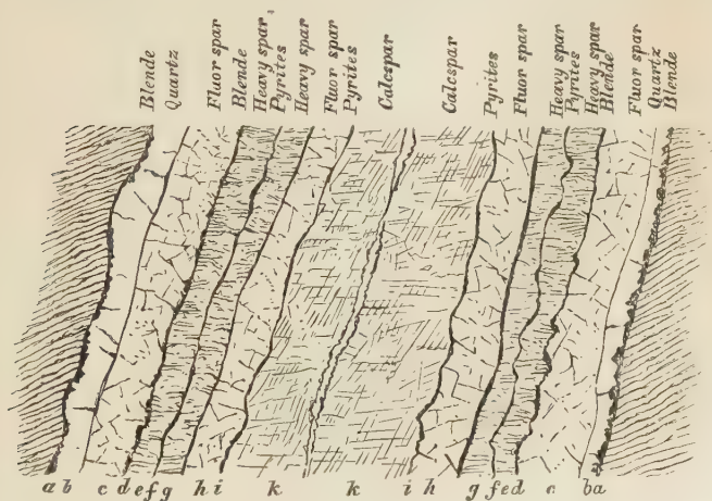
FIG. 39.—Section of the Drei Prinzen Spat Vein, near Freiberg; after v. Weissenbach.
